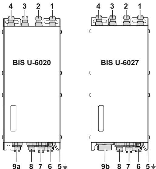
Figure 3: Electrical connection
